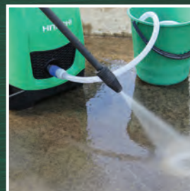
Step 6: Switch the washer off and connect the spray nozzle, switch the washer back on & pull the trigger to commence washing
