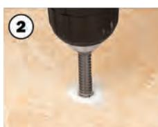
Once the hole has started, raise the drill gradually up to the vertical line
