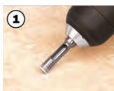
The drill needs to run before hitting the surface. To avoid sliding of the drill, start with an angle of 45°
