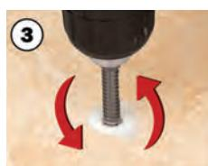
Make an oscillating movement while drilling
