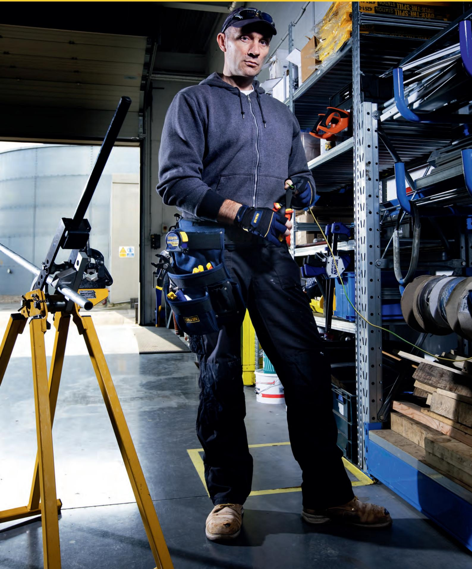
**Formers supported on both sides so they will not twist under heavy loading**
