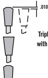
Triple Chip tooth grind combined
