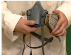
1. Line up the 3 indented lines on the inner side of the filter with the arrow on the half mask and push together.
