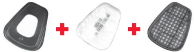
1. Place the white particulate filter (3M 5000 series) into the plastic retainer so that the printed side will face the gas & vapour filter, then put the gas and vapour filter on top and press firmly to click into place.
