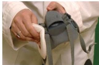
1. Align the filter bayonet fitting with the mask bayonet fitting.
