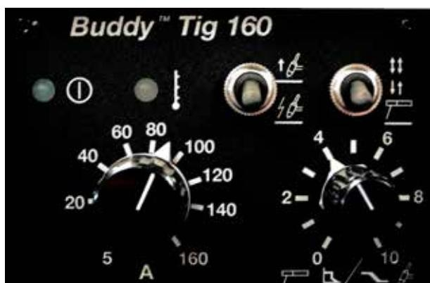
The control panel on the Buddy™ Tig 160 features one adjustment knob to set the weld current and one to set the slope down time in TIG mode or the arc force in MMA mode.
