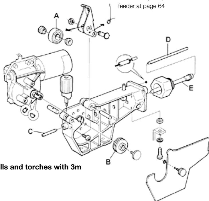
**Welding with aluminium wires. Use appropriate feeding rolls and torches with 3m cable.**
